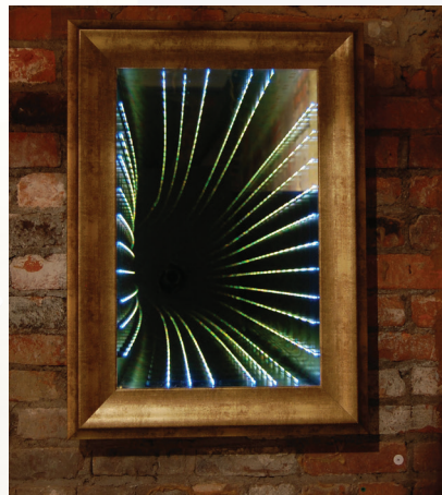
Infinity mirror using two way mirror
