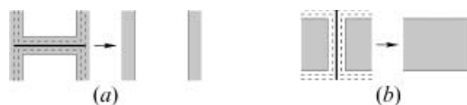
Figure 5. External scale-space events. (a) Opening: the thin horizontal connection is eliminated after the inward going segments meet. (b) Closing: the vertical gap is closed after the outward going segments meet; thick lines in (a) and (b): external scale-space event.
