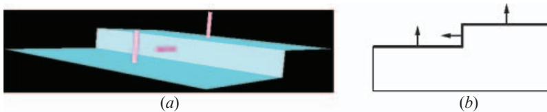
Figure 17. (a) Normals of stair in 3D (red cylinders) directly depend on (b) the polygon defining the neighbouring facet.
