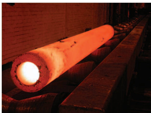
Figure 18 Inconel 740H pipe after extrusion (Shingledecker, 2012)
