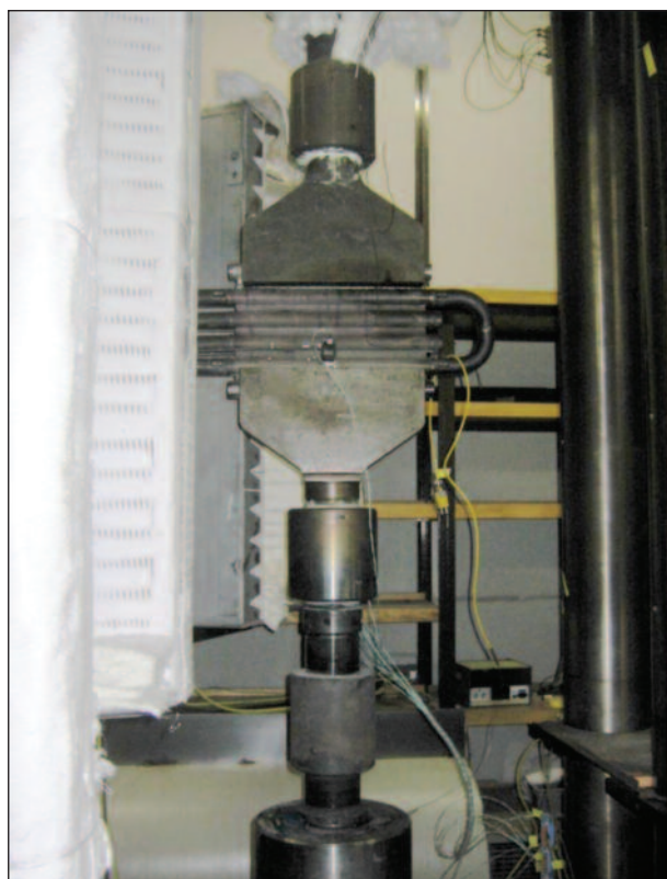
Figure 9 Testing of a membrane wall by Hitachi Power Europe (Jedamzik, 2012)
