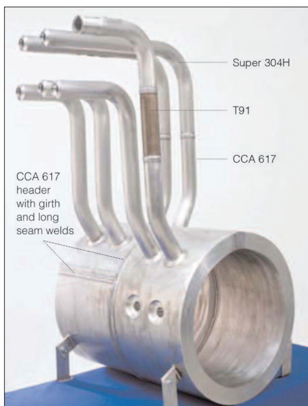
Figure 17 Mock-up header manufactured by Alstom USA (Viswanathan, 2008b)
