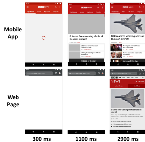
Figure 1: Comparing the mobile app and mobile web browser loading processes for BBC News over an LTE cellular network.
