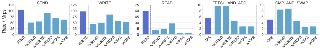
Figure 4: The contention of different data verbs on PU (NVIDIA). The leftmost bar on each subfigure is the request rate of running the victim only. The right 5 bars of each subfigure are the victim’s rate when the attacker is running.
