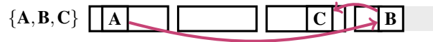
Figure 1: Key insertion in Aardvark consists of the following steps. (1) The key is inserted into the last slot of the dictionary. (2) Its predecessor is verified, and the new slot's next pointer is attached to the predecessor's next pointer. (3) Its predecessor's next pointer is updated to the inserted key. Observe that the operations shown here require only one update operation on a vector commitment (updating the predecessor's next pointer) since the tail is stored by the validator and not committed to.
