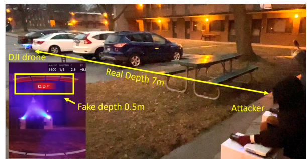
Figure 1: An attacker uses two projectors to launch DoubleStar at 7m away on a flying DJI drone. A fake depth of 0.5m is created by the attack and detected by the DJI drone as a real obstacle during the daytime.
