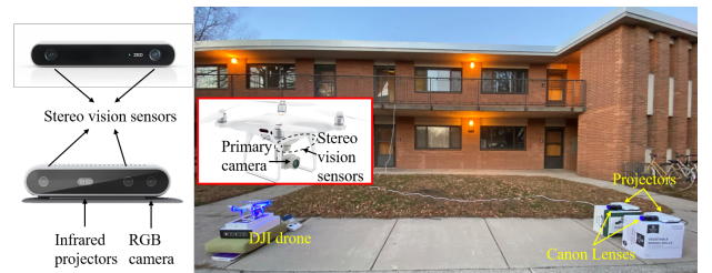
Figure 13: Outdoor attack experimental setup: the DJI drone is on the left and two Epson PowerLite 1771W projectors [11] combined with two Canon EF 75 – 300mm zoom lenses are on the right. We also conduct the experiments on ZED and RealSense in the experiments. All three attack devices have a pair of stereo vision sensors. The DJI drone has a primary camera at the bottom and RealSense has extra infrared projectors and an RGB camera.
