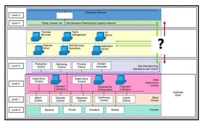
Refer to the exhibit. Which product must be positioned where the "?" is placed to connect these different network levels?
