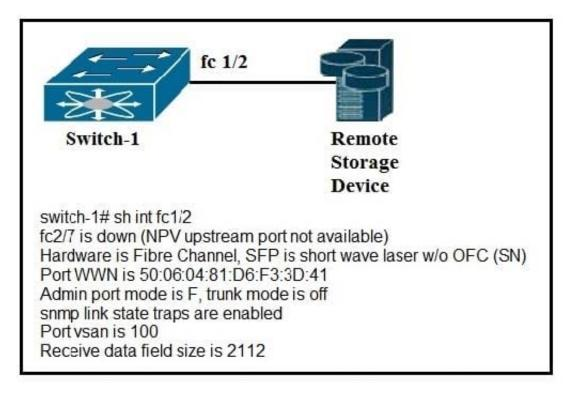
A remote device connected to fc 1/2 fails to come online. Which do you configure to resolve the issue?
