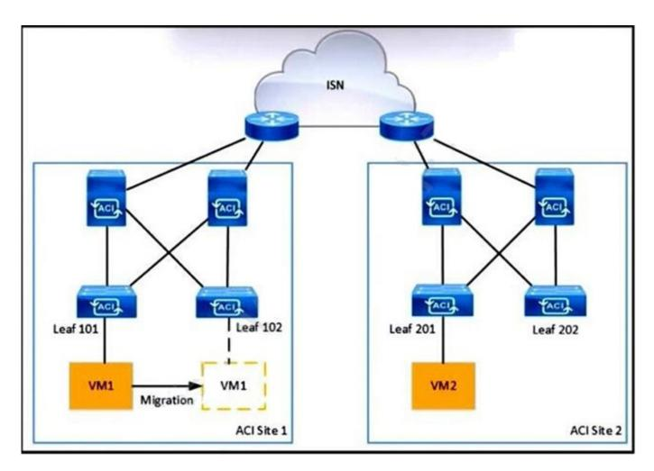
VM1 and VM2 are in Cisco ACI POD1 and communication takes place. Which event is triggered when VM2 is live migrated from POD1 to POD2?
