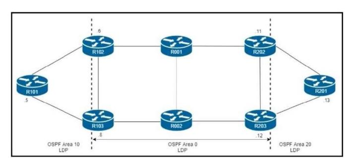
R101 is peering with R102 and R103, and R201 is peering with R202 and R203 using iBGP Labeled Unicast address families. The OSPF area 0 border routers are in a full iBGP Labeled Unicast mesh, and VPNv4 routes are exchanged directly between PE routers R101 and R201 through iBGP
