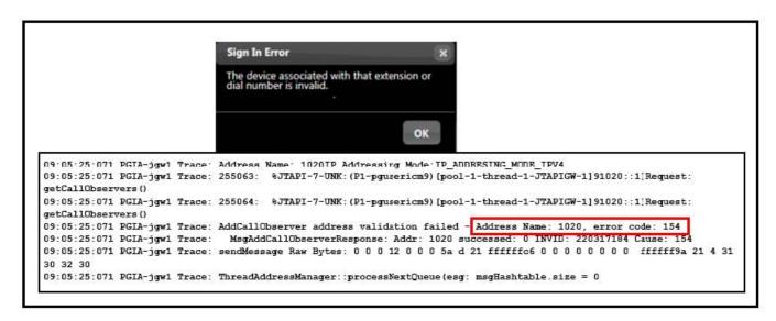
In a Cisco Finesse 10.0(x) deployment, an agent with single line 89XX hard phone is having trouble logging in to the desktop. The error message highlighted has been found in the PG jgw1 log file.
