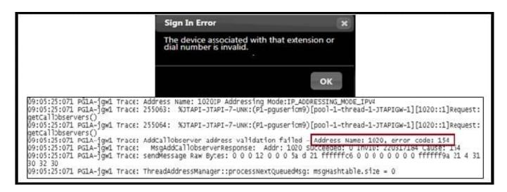
In a Cisco Finesse 10.0(x) deployment, an agent with single line 89XX hard phone is having trouble logging in to the desktop. The error message highlighted has been found in the Jgw1log file.
