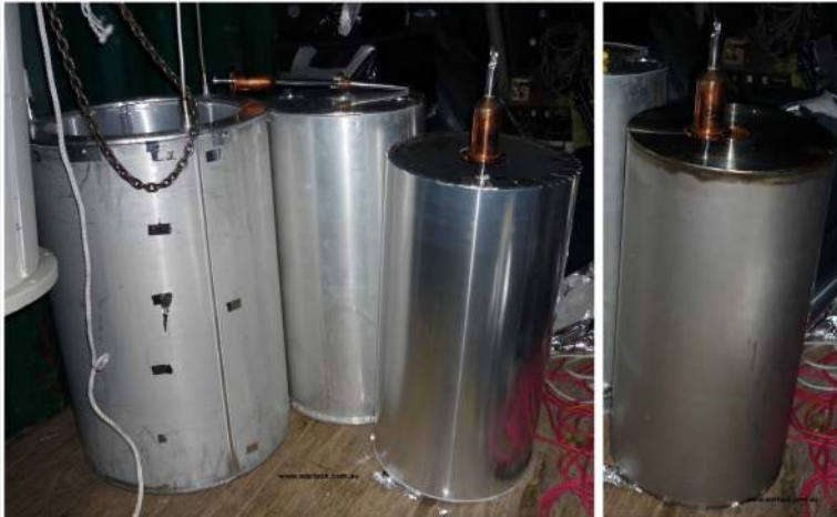
Figure 4. Left; The doughnut shaped 'Liquid Nitrogen Vessel' (left) is separated from the '20 K Radiation Shield' (middle) that covers the 'Liquid Helium Vessel' (right). Right; One layer of aluminium foil is removed to expose the stainless steel 'Liquid Helium Vessel'.
