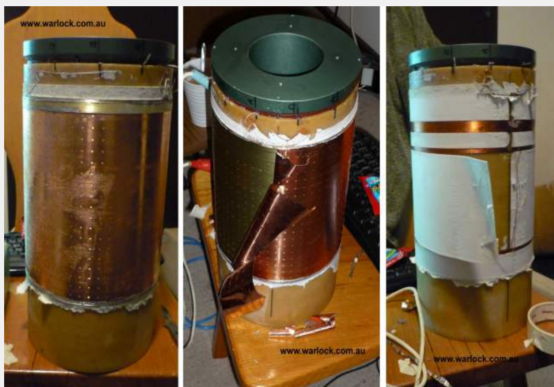
Figure 8. Left; After the first layer of 'Superconducting Wire' was removed it was de-soldered at the top. Underneath is a thin layer of copper foil that was removed. Middle; Underneath the copper foil is a second layer of 'Superconducting Wire' that was also unwound. Right; Under the second layer of 'Superconducting Wire' is a cardboard section that contains 3 copper coils (of varying size) wound around the 'Rare Earth Metal Core'.
