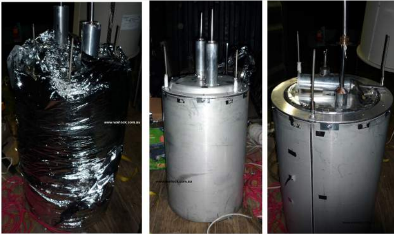
Figure 3. Left; The Mylar sheet was removed. Middle; The top plate is unscrewed from the 'Liquid Nitrogen Vessel'. Right; The filling tubes to the 'Liquid Helium Vessel' are thin stainless tube and break easily.
