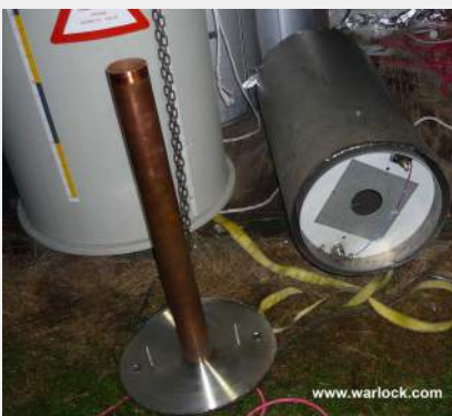
Figure 5. Left; The base of the 'Liquid Helium Vessel' is cut open with an angle grinder and the base with connected copper pipe is removed.
