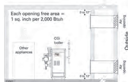
Figure 5 Air from outdoors — horizontal ducts
