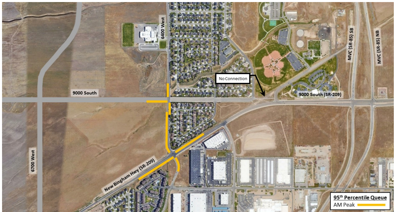
Figure 8: 95 th percentile queues along 6400 West during the morning peak hour with no-build mitigated conditions.
