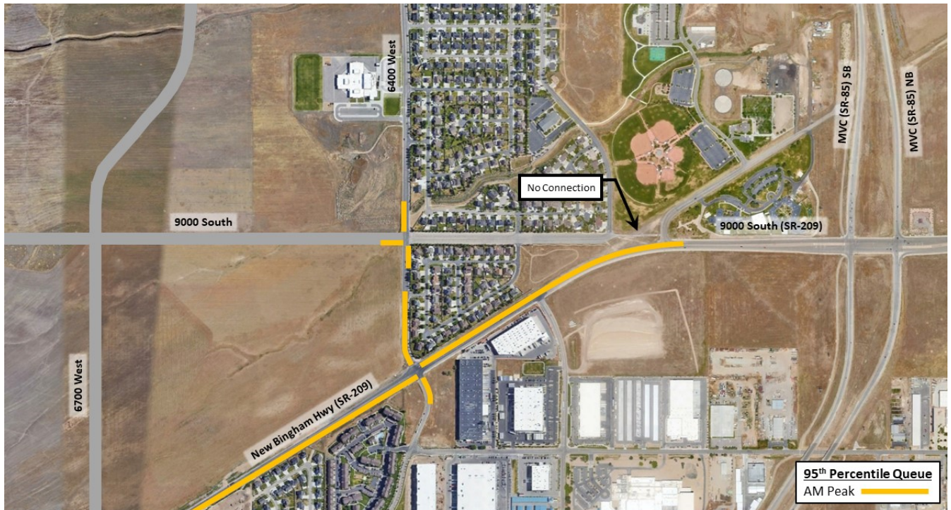
Figure 6: 95 th percentile queues along 6400 West during the morning peak hour with no-build conditions.
