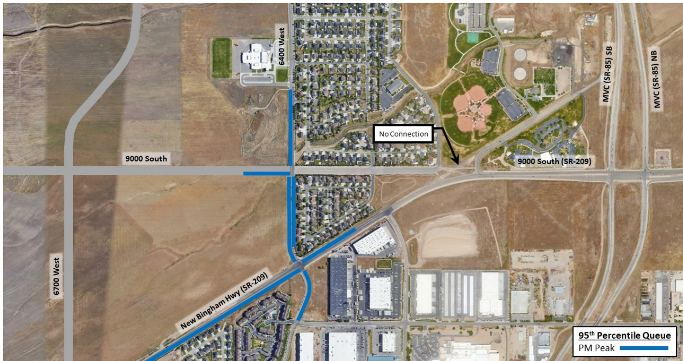
Figure 7: 95 th percentile queues along 6400 West during the evening peak hour with no-build conditions.
