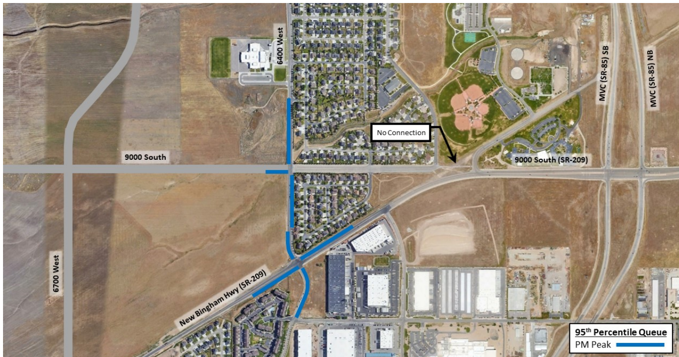
Figure 11: 95 th percentile queues along 6400 West during the evening peak hour with additional mitigation measures.
