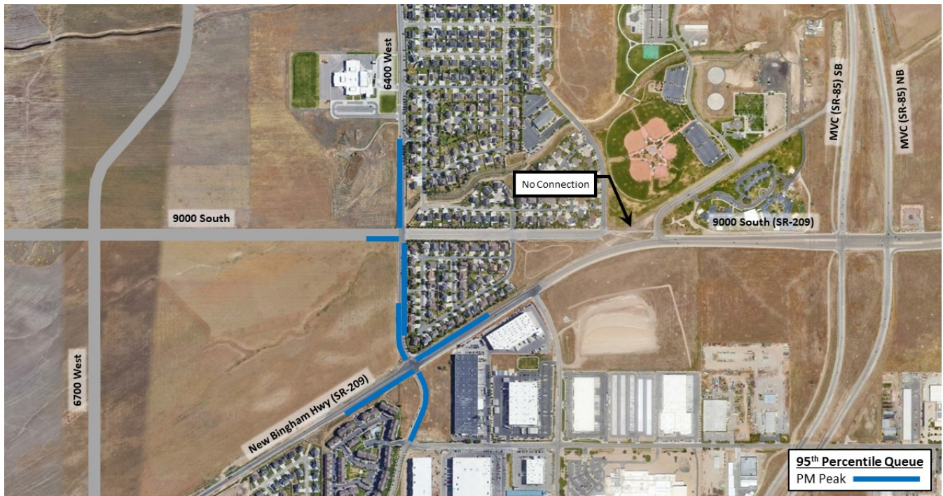
Figure 9: 95 th percentile queues along 6400 West during the evening peak hour with no-build mitigated conditions.
