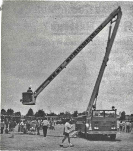
SEEKING TAKEOFF CLEARANCE . . . . Some spectators went for a ride in West Springfield's new snorkel, a hydraulically operated bucket which lifts firefighters to previously inaccessible heights.
