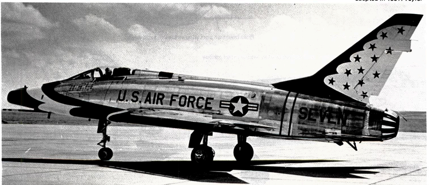
F-100D number SEVEN (the spare) shows several details to good advantage particularly the polished afterburner eyelids, identical size stars on tail, smoke probe, general high polish, 45 flag panel, and the pilot name panel adopted in 1967. Taylor
