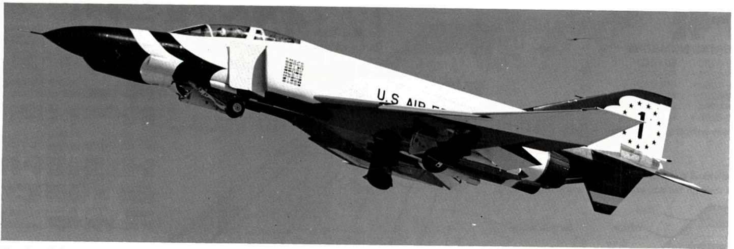
The first F-4E takes off for Nellis. Note the absence of underwing tip striping, and crew name blocks. Notice also the factory applied nose scallops which were quickly altered to give a more rakish, streamlined appearance.
