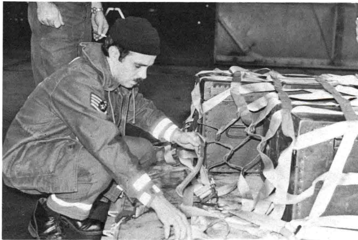
BATTENING DOWN . . . . . SSgt. Don Poudrier, 58 APS, cargo specialist, adjusts netting of palettized cargo prior to deployment.
