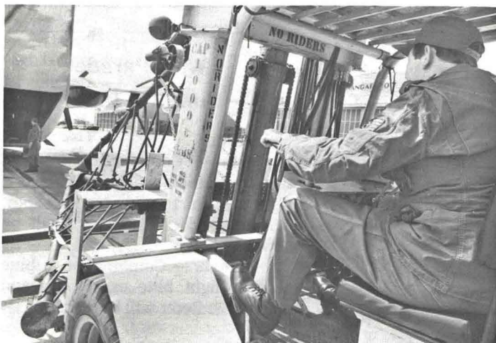
LOADING . . . . Driving a 10K fork lift, SSgt. Bruce MacRae, 58APS, eases a wing jack towards the open hatch of a 731 TAS bird.
