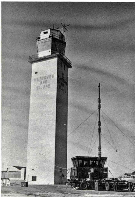
BIG BROTHER . . . . . Westover's control tower stands silent during its mobilization while a portable tower, an AN/TSW-7, takes over the chores.
