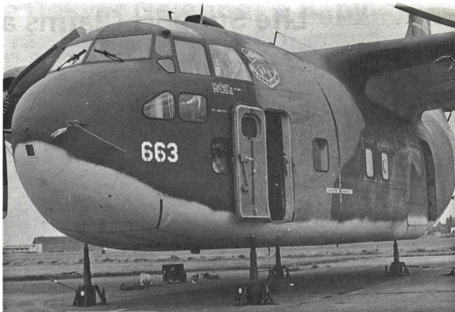
A Westover C-123 rests on jacks on the Wiesbaden AB flightline. Maintenance crews jacked up the transport to test its landing gear hydraulics.
