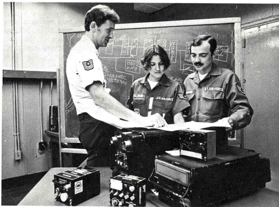
MSgt. Paul Fite, left, traces a circuit on a schematic diagram of the ARC-164, as SSgts. Janet Malouin and Donald Edwards look on. The ARC-164, left replaces the two large boxes at the right, the ARC-27 and ARC-34.
