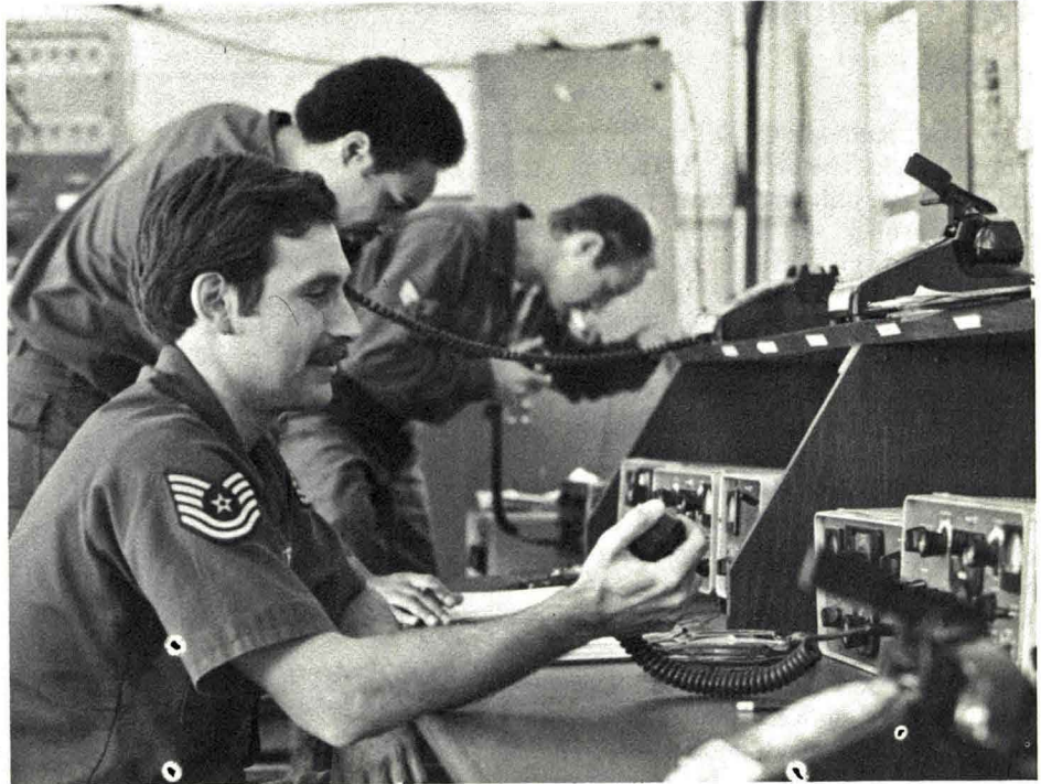
TSgt. Steven Leib , 901 CF training NCO, foreground; a member of the 1913 Comm. Sq., center; and Sgt. James Dester , also with the 901 CF, operate a KWM-2A transceiver at Langley AFB, Va.
