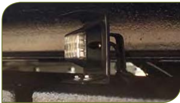
45° Horizontal or Vertical brackets and 90° Bracket optional for versatile mounting in any area on the vehicle
