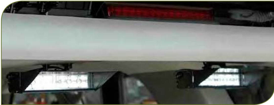
Dual Predator Lights mounted to the rear headliner in the back window of a Ford Explorer
