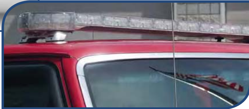
Clear lens with low profile fixed mount brackets
