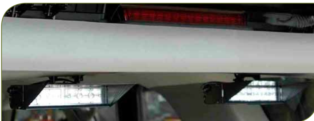
Predator Lights mounted to the rear headliner in the back window of a Ford Explorer
