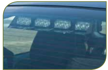
4 Module Suction Cup Mount mounted in the rear window of a Ford Mustang
