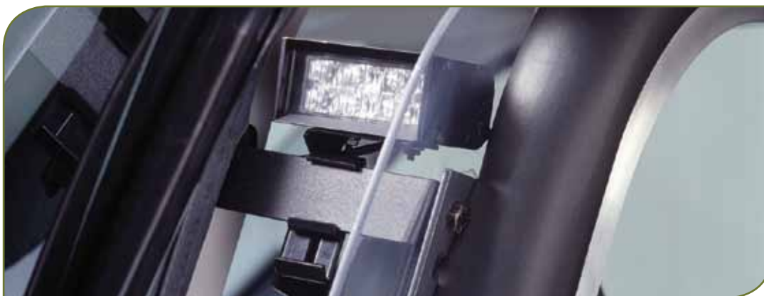
Single Windshield light mounted with optional Prisoner Screen Bracket (windshield shroud removed)
