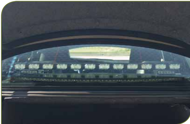
12 Module Bar mounted in the rear window of a 2011 Dodge Charger (no shroud)
