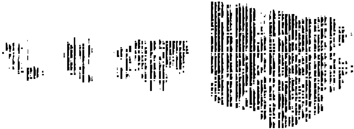
Figure 8.13.: Hardware utilisation of the specification LONG with sizes 1, 10, 100 and 1000 from left to right visualised in Xilinx Vivado manually edited to show only the actual specification without Xillybus and the input and output FIFOs. See Figures A.1 to A.4 in Appendix A.4 in the appendix for the entire visualisations as generated by Xilinx Vivado.
