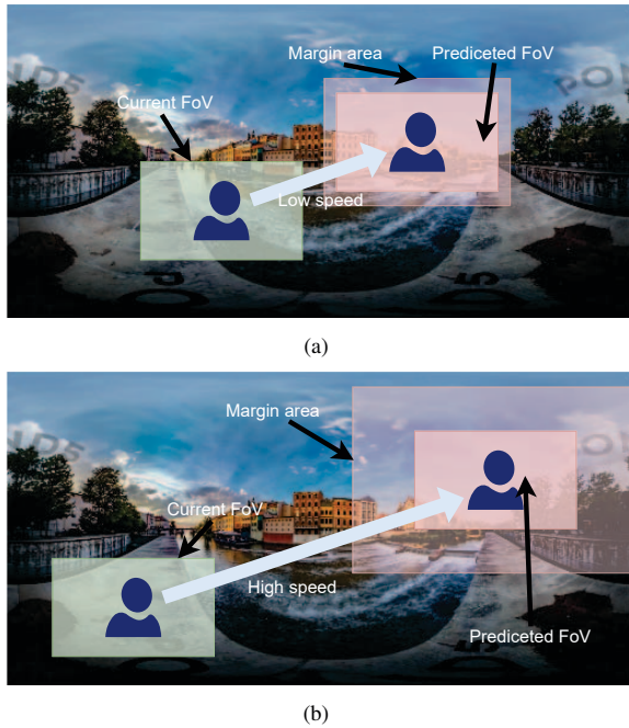
Fig. 6. Dynamic margin area frames based on gaze tracking: (a) smaller margin area with low gaze movement speed; (b) larger margin area with high gaze movement speed
