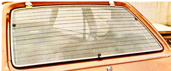
● A. Rear window electric defogger (includes 51-amp alternator and rear window tinted glass)
