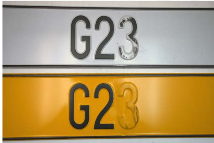
Samples post fuel - ink removed from embossing/letters
