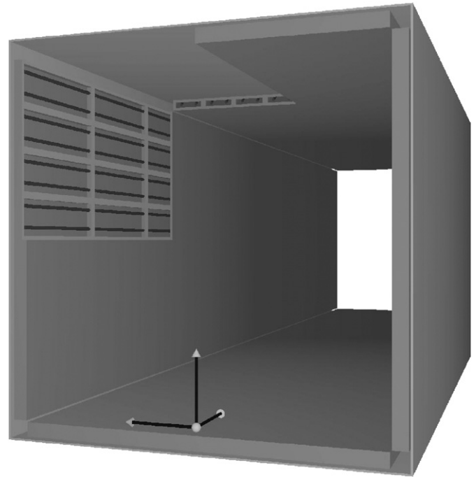
Fig. 15. Screen capture of MCNP model of the large area neutron detection system consisting of 320 two-tube detector assemblies. The cutaway shows the arrangement of tubes in the assembly. The coordinate vectors shown are 1 m long.
