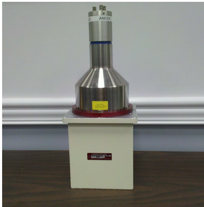
Figure 4: Photo of one of the EJ-309 liquid scintillator detectors.
