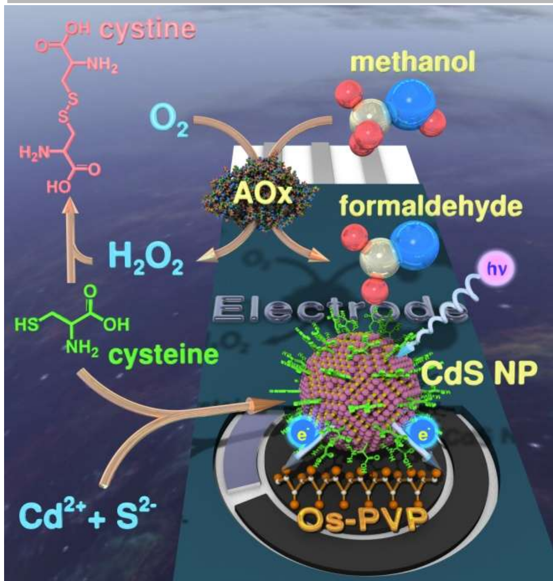
Scheme 1. Photoelectrochemical assay for methanol through detection of CdS QDs “wired” by an Os-PVP complex to the surface of a screen-printed carbon electrode.
