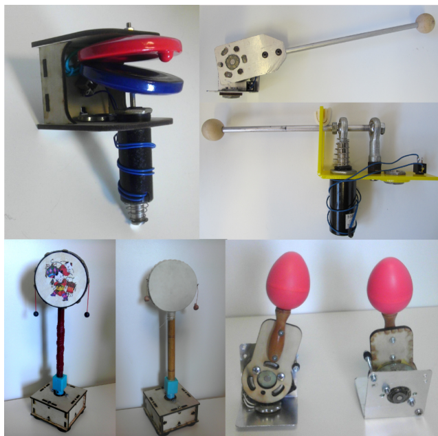
Figure 1: The array of solenoid-based instruments used in this project. Top-left: Castanet, Top-right: Rotary solenoid-based striker, Mid-right: Linear solenoid-based striker, Bottom-left: Rattle Drums, Bottom-right: Egg Shakers.
