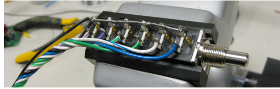
Figure 8. Input wiring of pot
