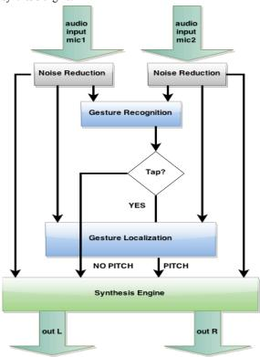
Figure 1. Signal flow for the described system.
