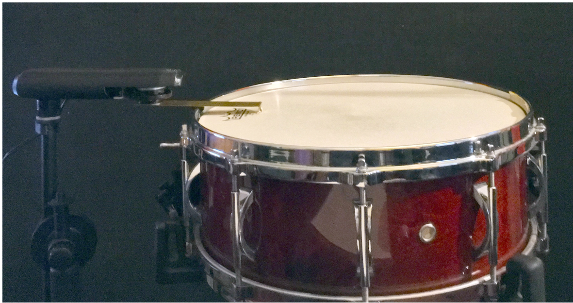
Figure 2: DRMMR in the stand mounted configuration with a snare drum.
