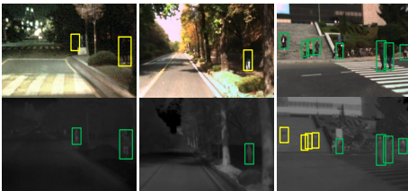
Figure 1: Yellow bounding boxes indicate detection failures with one image channel.
