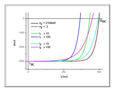
Everything else has been kept simple - no shunt or series resistors. This means that the shunt resistance  $R_{SH}$  is very large ("infinity"),  $R_{SE}$  is zero. The ideality factor of the second diode is  $n_2 = 2$  or n = 3 (the ideality factor of the first diode is always  $n_1 = 1$  by definition), and the two pre-exponential factors are  $l_1 = 0,1 \mu A$  and  $l_2 = 10 \mu A$  as starting values once more, but also 10 times and 100 times that number. The photo current is 3 A.
