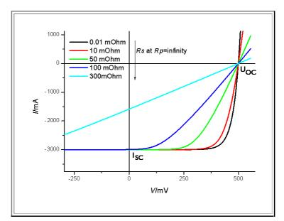
Everything else has been kept "ideal". This means that the shunt resistance *R*<sub>SH</sub> is very large ("infinity"), the ideality factor of the second diode is *n* = 2, and the two pre-exponential factors are *l*<sub>1</sub> = 0,1 μA and *l*<sub>2</sub> = 10 μA. The photo current is 3 A.
